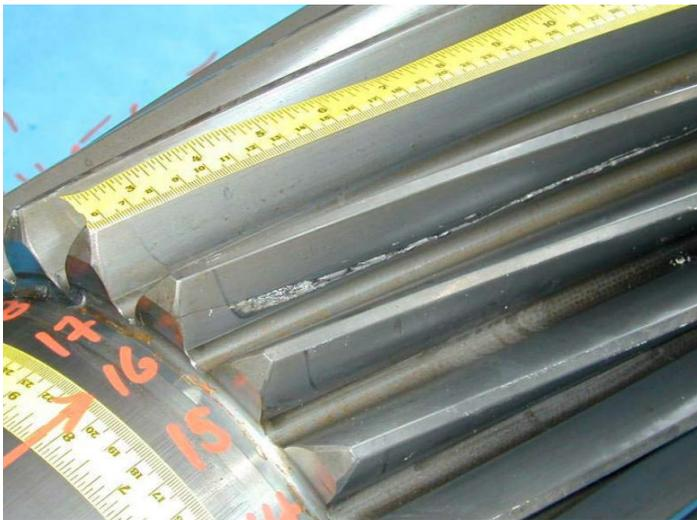
Gearbox teardown shows cracked tooth #16
